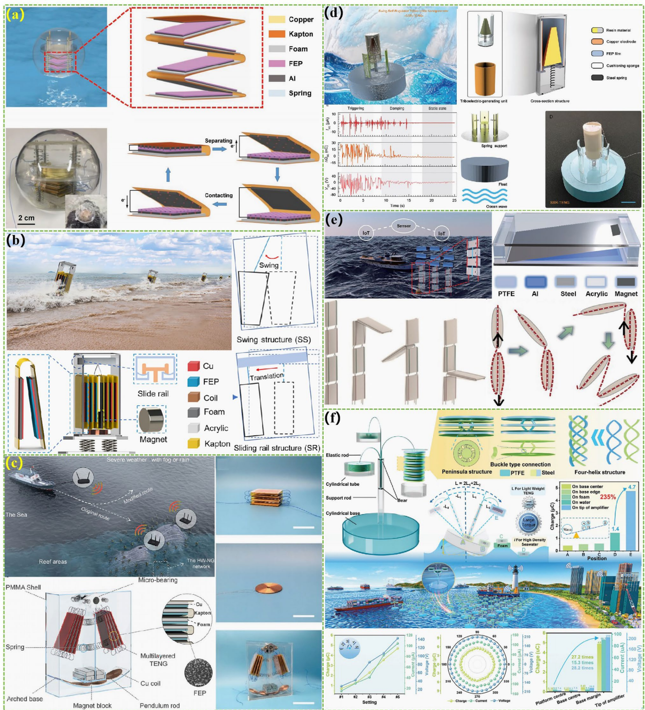
Fig. 11 Spring-assisted TENGs for the marine energy harvesting. a A high-output wave energy harvesting TENG using a spring, guideway, and multilayer structure. Reproduced with permission from Ref. [123]. Copyright 2018, Wiley–VCH. b The swinging TENG by installing a spring base at the bottom. Reproduced with permission from Ref. [156]. Copyright 2022, American Chemical Society. c The multilayer structure TENG with the assisted springs and the swinging magnet. Reproduced with permission from Ref. [175]. Copyright 2021, Wiley–VCH. d A self-adjusting oscillation TENG based on a dual spring coupling system. Reproduced with permission from Ref. [176]. Copyright 2023, Wiley–VCH. e An elastic TENG based on cantilever beam. Reproduced with permission from Ref. [177]. Copyright 2023, Springer Nature. f TENG with the amplitude amplifier constructed by the elastic rod. Reproduced with permission from Ref. [129] Copyright 2024, Wiley–VCH
