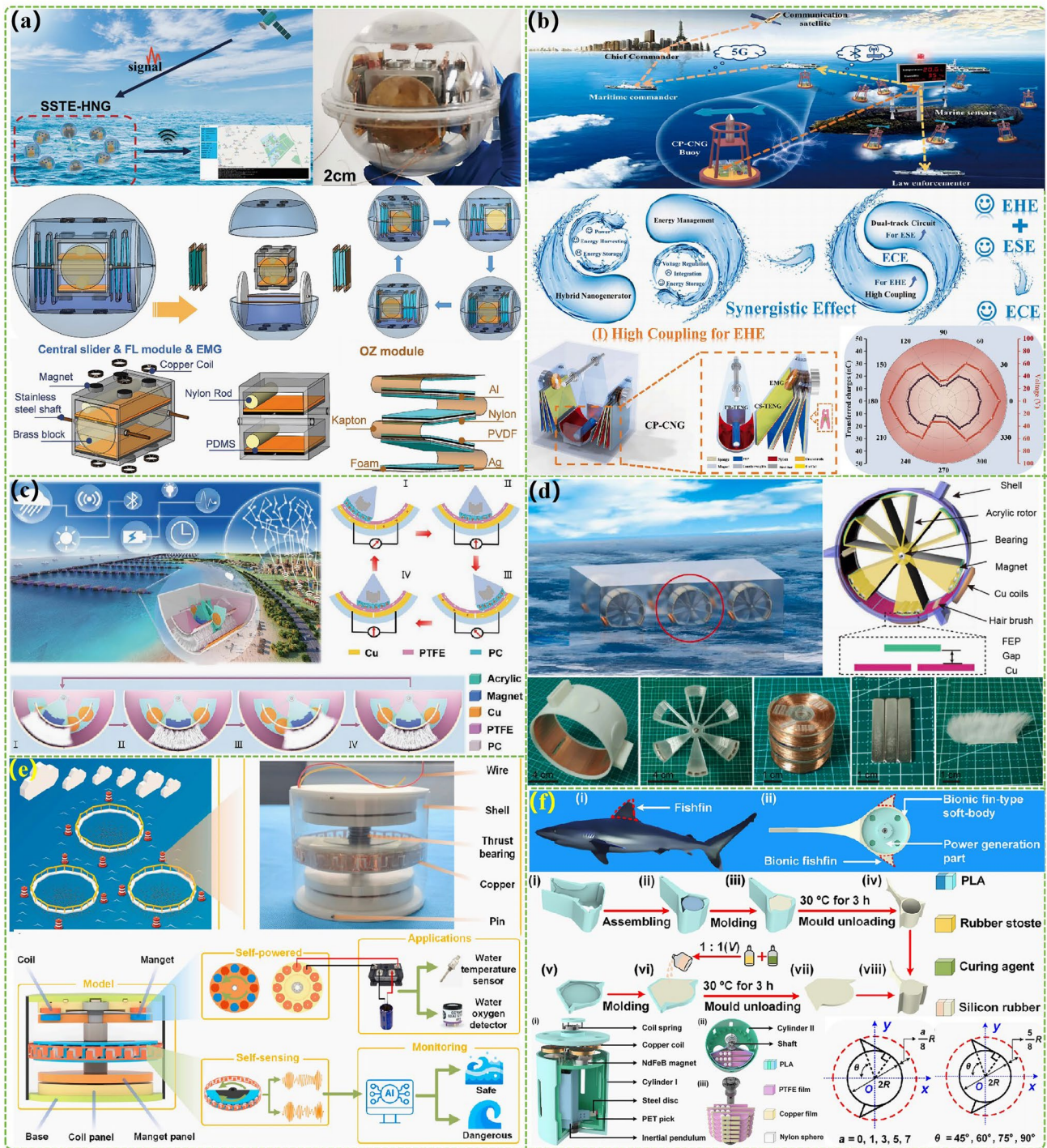
Fig. 10 Hybrid generators for the marine energy harvesting. a Hybrid generators obtained by simple integration of different types of generators. Reproduced with permission from Ref. [148]. Copyright 2022, The Royal Society of Chemistry. b A triboelectric-electromagnetic hybrid generator with swinging structure. Reproduced with permission from Ref. [157]. Copyright 2024, Elsevier. c The hybrid generator based on the pile and Halbach array. Reproduced with permission from Ref. [159]. Copyright 2022, Wiley-VCH. d A hybrid generator composed of soft contact cylindrical TENG and swinging structure EMG. Reproduced with permission. from Ref. [161]. Copyright 2019, Elsevier. e A hybrid rotary generator through eccentric pendulum and rectification enhancement mechanism. Reproduced with permission from Ref. [162]. Copyright 2024, Elsevier. f A flexible biomimetic fin hybrid generator with a swinging rotating structure. Reproduced with permission from Ref. [163]. Copyright 2022, American Chemical Society
