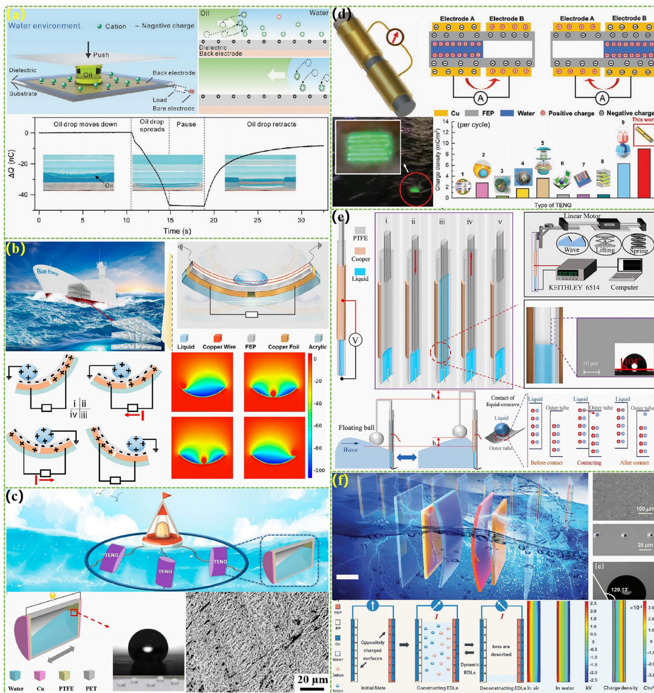
Fig. 5 Liquid–solid TENGs for harvesting the marine energy. a Liquid–solid TENG with the oil phase. Reproduced with permission from Ref. [79] Copyright 2022, Wiley–VCH. b The high-output liquid–solid TENG with the seawater. Reproduced with permission from Ref. [81] Copyright 2020, American Chemical Society. c Liquid–solid TENG with the instantaneous contact structure. Reproduced with permission from Ref. [82] Copyright 2021, Elsevier. d Tube liquid–solid TENG with the high charge volume density. Reproduced with permission from Ref. [83] Copyright 2021, Wiley–VCH. e Liquid–solid TENG with the curvature effect. Reproduced with permission from Ref. [85] Copyright 2023, Elsevier. f A liquid–solid TENG based on a reverse dynamic double-layer structure. Reproduced with permission from Ref. [86] Copyright 2023, Wiley–VCH
