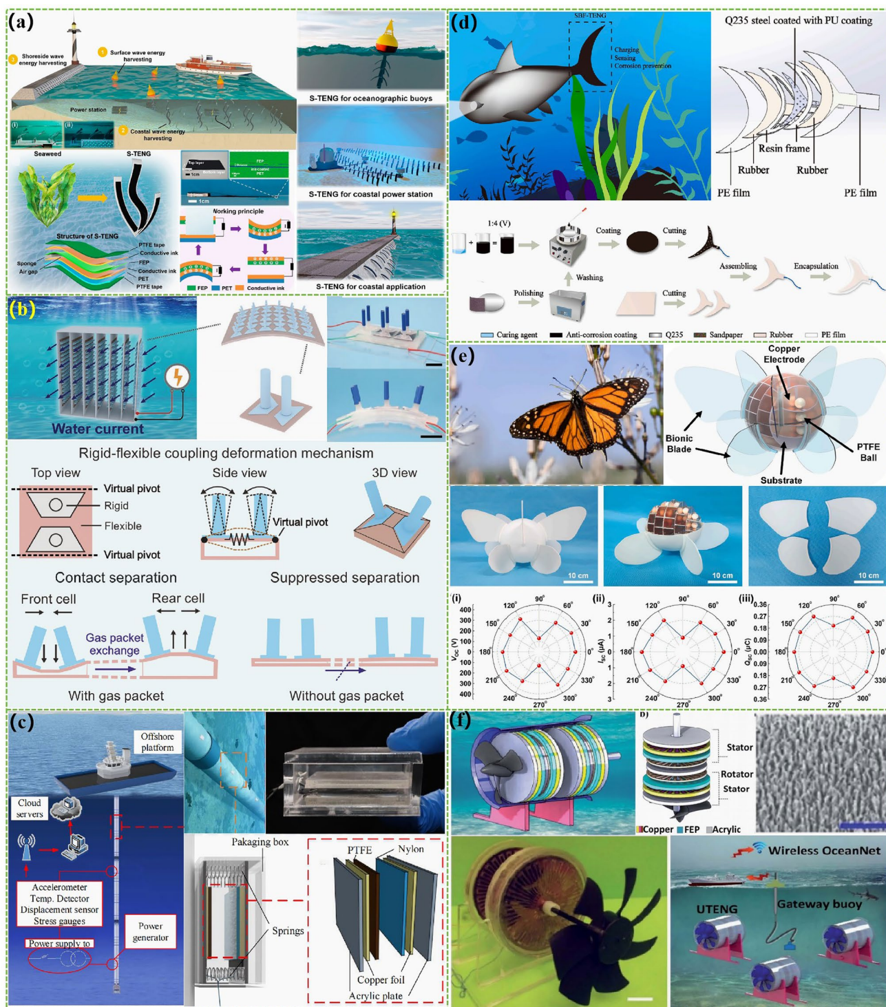
Fig. 17 Researches of undersea energy harvesting TENG. a An undersea energy harvesting TENG with biomimetic seagrass structure. Reproduced with permission from Ref. [228] Copyright 2021, American Chemical Society. b An undersea eddy current energy harvesting TENG. Reproduced with permission from Ref. [229] Copyright 2022, Wiley-VCH. c Undersea pipeline vibration energy harvesting TENG. Reproduced with permission from Ref. [230] Copyright 2019, MDPI AG. d Undersea energy harvesting TENG with biomimetic fish fin structure. Reproduced with permission from Ref. [233] Copyright 2023, Elsevier. e An undersea energy harvesting device consisting of biomimetic butterfly wings and TENG units. Reproduced with permission from Ref. [234] Copyright 2022, Elsevier. f An underwater TENG to obtain electricity from the power of currents. Reproduced with permission from Ref. [235] Copyright 2022, The Royal Society of Chemistry
