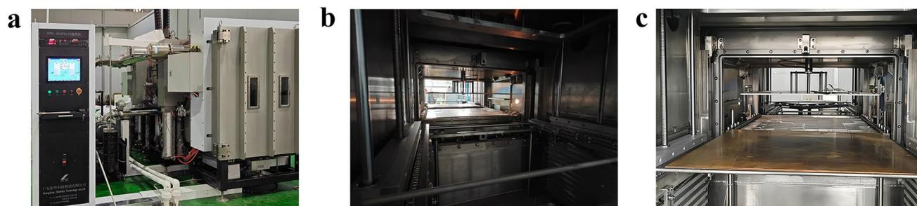
**Fig. 4** **a** Large-scale production equipment. **b** Internal structure of the deposition chamber. **c** RF electrode of large-scale production equipment
