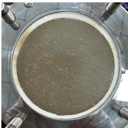
Fig. S1 Digital image of AgNWs on PTFE filter membrane after positive pressure filtration
