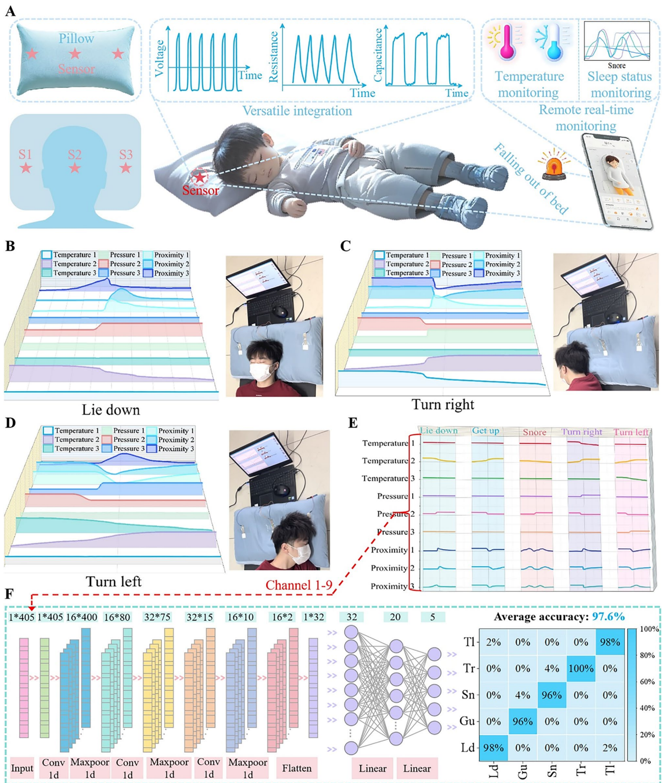
Fig. 6 A multimodal sensor-integrated system applied to human sleep monitoring. A Three multimodal sensors are placed at different positions on the pillow to prevent potential health risks. B Signal response of multimodal sensors when the body lies down. C Signal response of multimodal sensors when the body turns to the right side. D Signal response of multimodal sensors when the body turns to the left side. E Sensor signal changes in five sleep states: lying down, getting up, snoring, turning to the right, and turning to the left. F Five different sleep states are trained using 1D CNN with a recognition success rate of 97.6%
