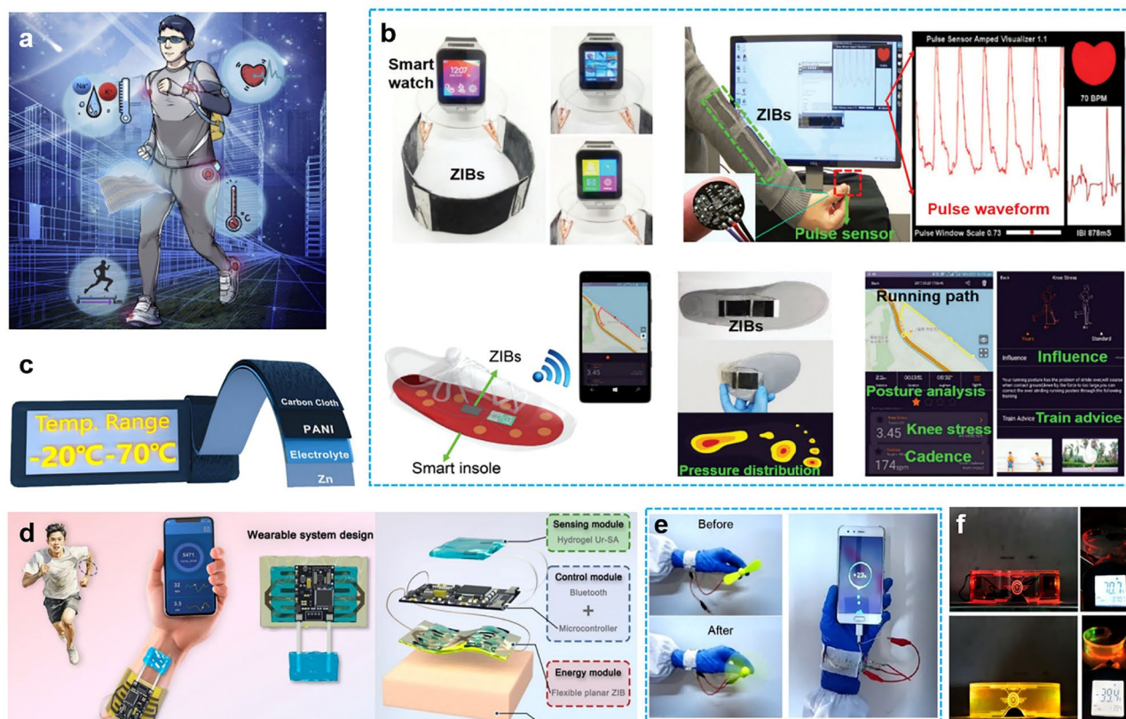
Fig. 13 a Schematic illustration of the rechargeable smart textile and an autonomous body area electronics network based on functional HEs. Reproduced with permission from Ref. [112]. Copyright 2020, Elsevier. b Three RZIBs were connected in series to power a commercial smart watch; Four RZIBs were integrated in series to power a pulse sensor; Two ZIBs were connected in series to operate the smart insole; Optical photograph of the RZIBs-powered smart insole (top), the bending status of the smart insole (middle) and the pressure distribution when standing on the insole (bottom); and Running path (left) and the sport analysis results (right) obtained from the RZIB-powered smart insole. Reproduced with permission from Ref. [53]. Copyright 2018, Royal Society of Chemistry. c Illustration of the ZBL electrolyte-based ZIBs with extended lifespan across -20 to 70 °C. Reproduced with permission from Ref. [100]. Copyright 2024, Wiley-VCH. d Schematic illustrations of the biocompatible Ur-SA-based RZIBs: Ur-SA hydrogels are fabricated with the properties to apply to flexible planar cells, and the superior biocompatibility of Ur-SA as the sensor makes real-time physiological signals and human movements detection possible, powered by Ur-SA-based flexible planar cells. e Three series-connected fiber RZIBs can power a fan and charge a mobile phone when wearing on a human wrist. Reproduced with permission from Ref. [65]. Copyright 2024, Royal Society of Chemistry. f Demonstration of electronic devices powered by three pouch cells in series at -40 and 70 °C. Reproduced with permission from Ref. [82]. Copyright 2024, Nature Publishing Group
