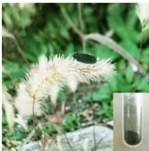
Fig. S6 Optical image of a piece of sample made from the as-synthesized WS 2 -rGO heterostructure nanosheets, which is put on a Setaria viridis . The inset displays the image of the as-synthesized WS 2 -rGO powders
