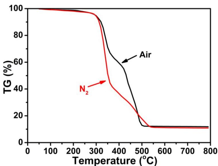
**Fig. S1** TGA plot of the metal-oleate complex precursor under N<sub>2</sub> and air atmospheres
