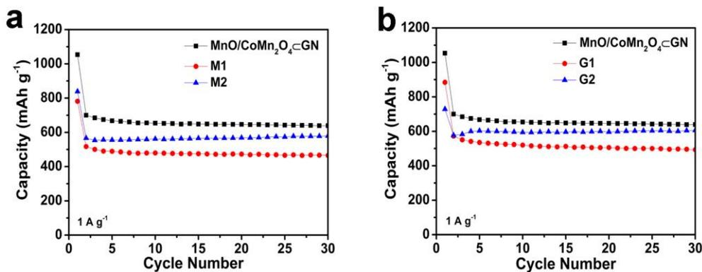
**Fig. S8** Cycling performances of MnO/CoMn<sub>2</sub>O<sub>4</sub>@GN, M1, M2, G1, and G2 at a current density of 1 A g<sup>-1</sup>
