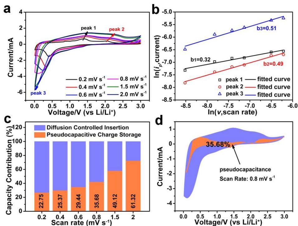
**Fig. S10** **a** CV profiles of the pure CoMn<sub>2</sub>O<sub>4</sub> electrodes at different scan rates with the potential range between 0.01 and 3.0 V. **b** The fitted lines and  $\ln(i_p)$  versus  $\ln(v)$  plots at different oxidation and reduction states. **c** The percentages of pseudocapacitive contribution at different scan rates. **d** Pseudocapacitive (red) and diffusion-controlled (blue) contribution to the charge storage of CoMn<sub>2</sub>O<sub>4</sub> at 0.8 mV s<sup>-1</sup>
