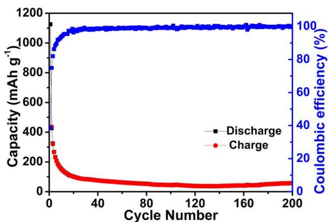
**Fig. S7** Cycling performance and coulombic efficiency of pure  $\text{CoMn}_2\text{O}_4$  at a current density of  $0.1 \text{ A g}^{-1}$
