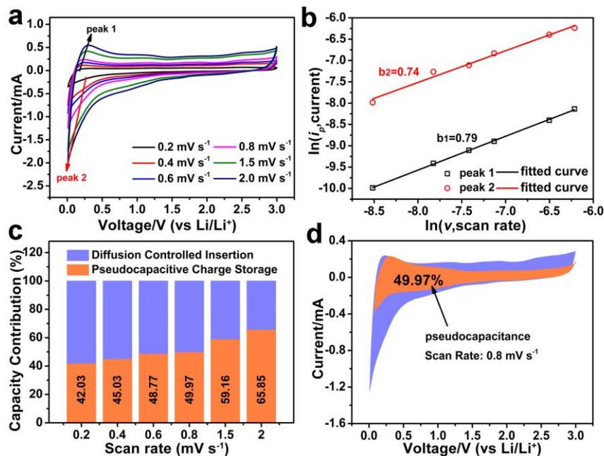
**Fig. S11** **a** CV profiles of the rGO electrodes at different scan rates with the potential range between 0.01 and 3.0 V. **b** The fitted lines and  $\ln(i_p)$  versus  $\ln(v)$  plots at different oxidation and reduction states. **c** The percentages of pseudocapacitive contribution at different scan rates. **d** Pseudocapacitive (red) and diffusion-controlled (blue) contribution to the charge storage of rGO at  $0.8 \text{ mV s}^{-1}$
