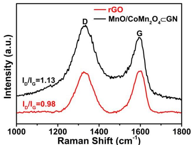
Fig. S2 Raman spectra of MnO/CoMn<sub>2</sub>O<sub>4</sub>@GN and rGO
