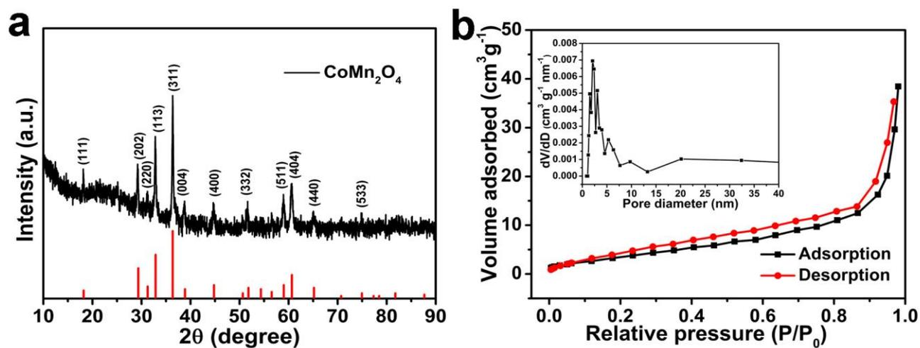
Fig. S4 **a** XRD pattern of the CoMn<sub>2</sub>O<sub>4</sub>. **b** Nitrogen adsorption-desorption isotherms and the pore size distribution curve of the CoMn<sub>2</sub>O<sub>4</sub>
