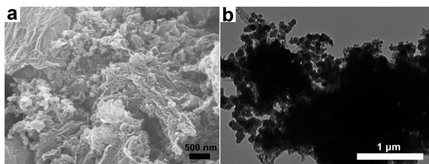
**Fig. S9** **a** SEM and **b** TEM images of MnO/CoMn<sub>2</sub>O<sub>4</sub>@GN after 150 cycles at 0.1 A g<sup>-1</sup>
