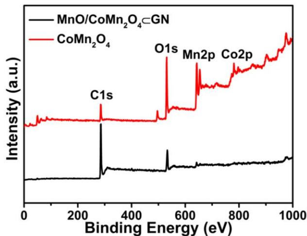
**Fig. S5** XPS spectra of the  $\text{CoMn}_2\text{O}_4$  and  $\text{MnO}/\text{CoMn}_2\text{O}_4@\text{GN}$  samples
