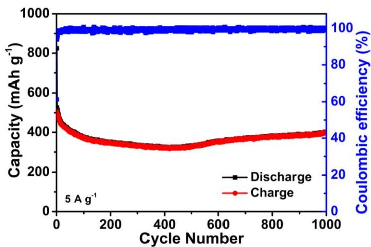
**Fig. S6** Cycling performance and coulombic efficiency of  $\text{MnO}/\text{CoMn}_2\text{O}_4@\text{GN}$  at a current density of  $5 \text{ A g}^{-1}$
