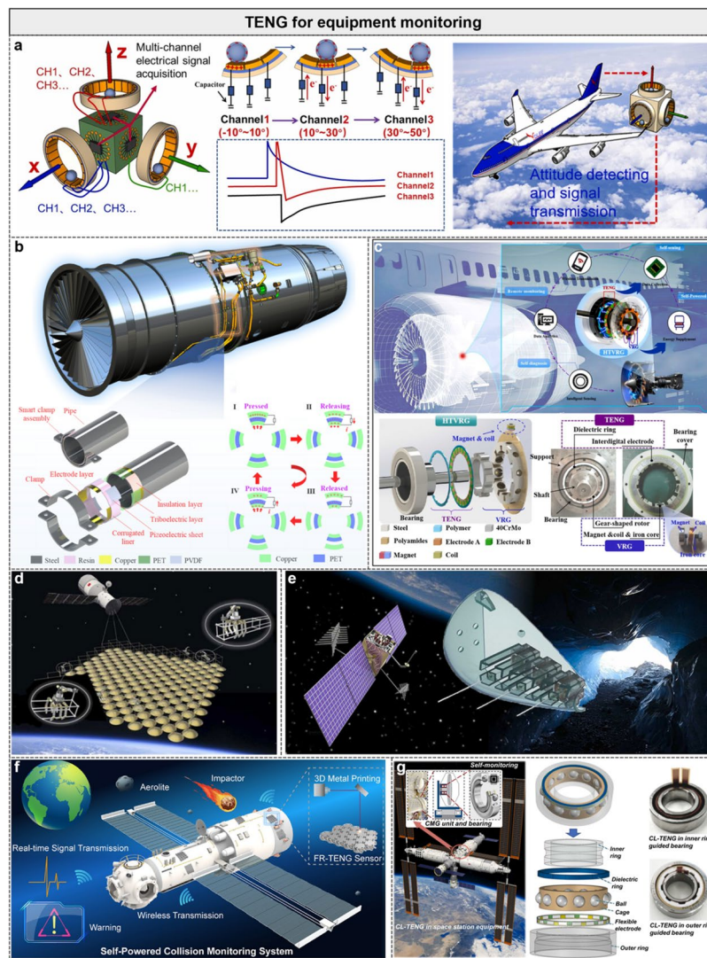
Fig. 9 TENG for equipment monitoring. a Design diagram and working schematic of a multi-channel self-powered sensor. Reproduced with permission from Ref. [215]. Copyright 2023, Elsevier. b Structural design and operating mechanisms of TPPC. Reproduced with permission from Ref. [216]. Copyright 2025, Elsevier. c Application prospects and structure of the HTVRG. Reproduced with permission from Ref. [217]. Copyright 2025, Elsevier. d Schematics of scalable self-attaching/assembling robotic cluster system. Reproduced with permission from Ref. [218]. Copyright 2022, Elsevier. e Application of BMWS for satellite surface feature acquisition in dark environments. Reproduced with permission from Ref. [219]. Copyright 2023, Elsevier. f Design and concept of the robust but flexible FR-TENG array is inspired by hexagon and pangolin scales. Reproduced with permission from Ref. [220]. Copyright 2023, American Chemical Society. g Application background and structure of the bearing-based CL-TENG. Reproduced with permission from Ref. [221]. Copyright 2024, Elsevier
