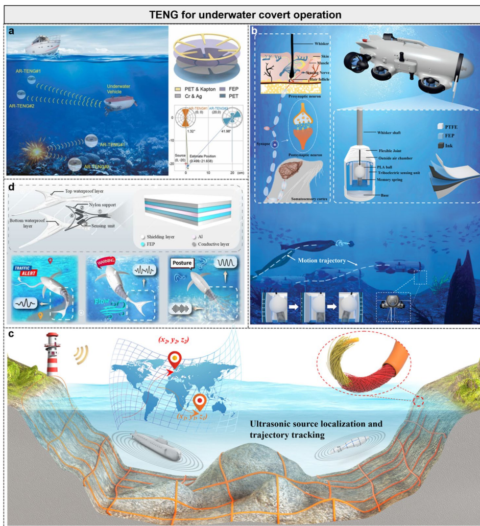
Fig. 7 TENG for underwater covert operation. a A self-powered angle-resolved triboelectric nanogenerator. Reproduced with permission from Ref. [189]. Copyright 2023, Elsevier. b A bionic underwater triboelectric whisker sensor array. Reproduced with permission from Ref. [190]. Copyright 2024, Wiley–VCH. c Schematic representation of a self-powered ultrasonic source localization and trajectory tracking system, incorporating multiple MTAS units deployed in the ocean. Reproduced with permission from Ref. [121]. Copyright 2025, American Chemical Society. d Working principles, structures, and application of the biomimetic tail fin sensor. Reproduced with permission from Ref. [191]. Copyright 2026, Elsevier
