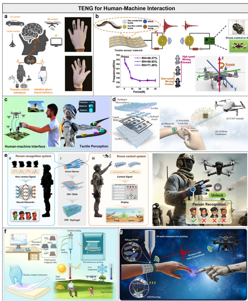
Fig. 6 TENG for human–computer interaction. a Minimalist design of a glove-based HMI based on the TENGs in two configurations. Reproduced with permission from Ref. [182]. Copyright 2019, Elsevier. b Wireless TENG system for car control and drone control in VR based on an RLC circuit. Reproduced with permission from Ref. [183]. Copyright 2020, Elsevier. c Application scenarios of BHES as a human–machine interaction interface. Reproduced with permission from Ref. [184]. Copyright 2023, American Chemical Society. d Stretchable triboelectric touch pad structure and an intelligent human–machine interaction system. Reproduced with permission from Ref. [185]. Copyright 2024, Elsevier. e PSP-TENG is integrated into smart gloves and its application scenarios in face-to-face recognition and drone control. Reproduced with permission from Ref. [186]. Copyright 2024, Wiley–VCH. f Realize HMI through CQAS/ZnO thin films and promote the development of drones. Reproduced with permission from Ref. [187]. Copyright 2025, Wiley–VCH. g Design and conceptual illustration of MXTENG-RFS. Reproduced with permission from Ref. [188]. Copyright 2025, Elsevier
