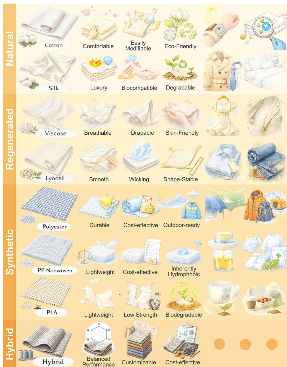
Fig. 7 Textile substrates for photothermal superhydrophobic modification: intrinsic properties and representative application scenarios. PLA: polylactic acid. PP: polypropylene
