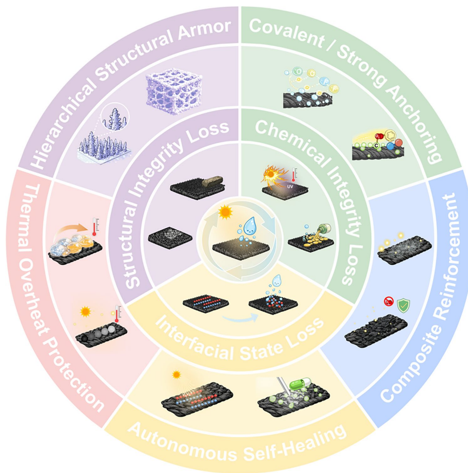
Fig. 19 Durability-oriented design framework for photothermal superhydrophobic textiles: failure pathways and corresponding reinforcement strategies
