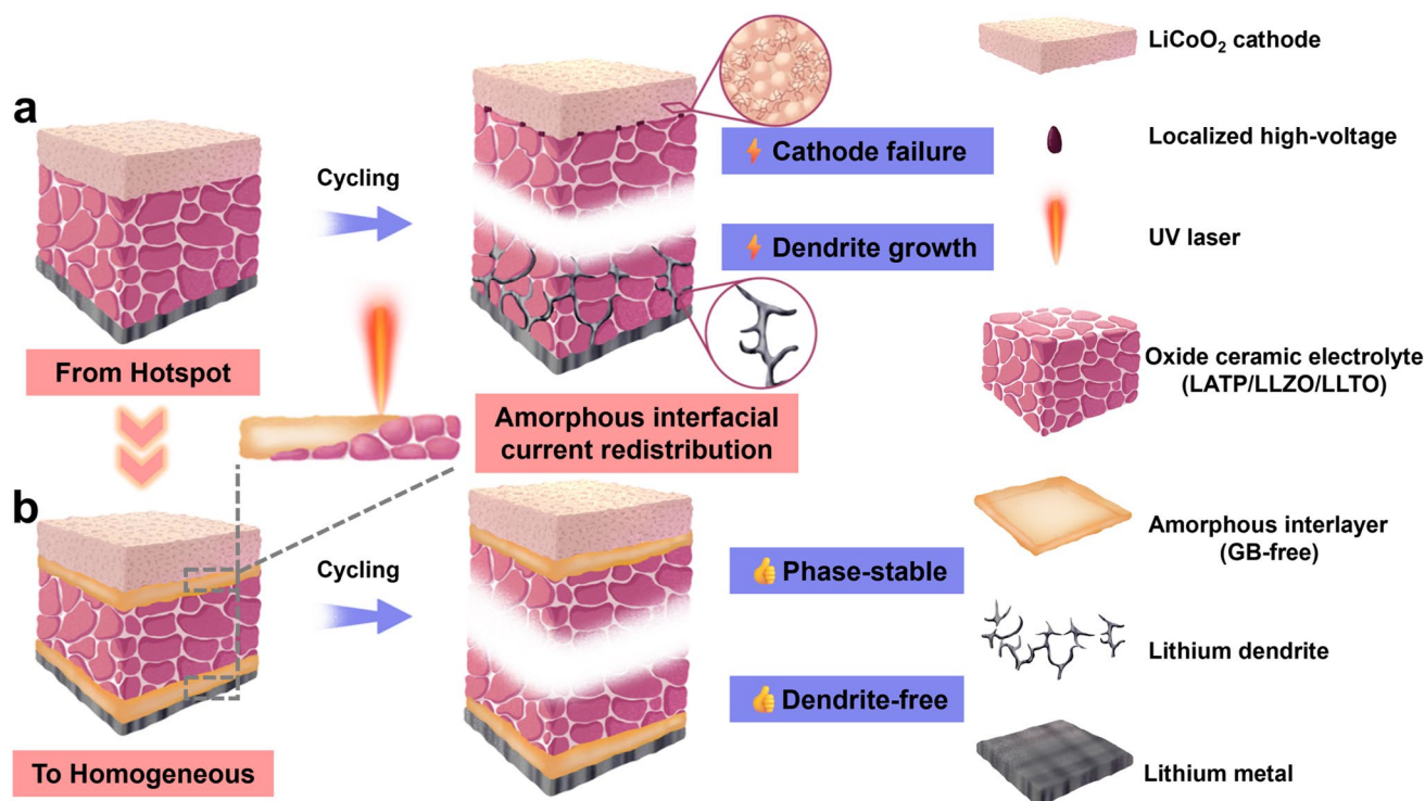
Fig. 1 Schematic illustration of the amorphous interfacial current redistribution strategy, achieving the transition from hotspot to homogeneous in polycrystalline OCEs. a Hotspot stage: Pristine OCE exhibits localized overpotentials at the electrolyte-cathode interface induced by surface GBs, leading to structural degradation in part of the cathode. At the electrolyte-anode interface, dendrites infiltrate from the surface GBs. b Homogeneous stage: The laser-engineered amorphous interlayer eliminates surface GBs, achieving homogeneous current distribution and stable interfaces
