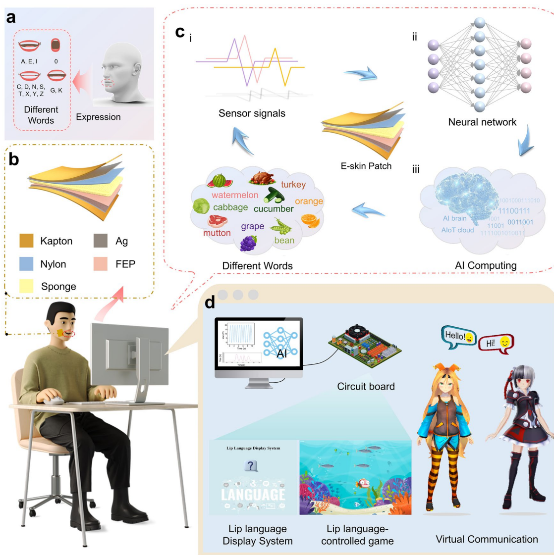
Fig. 1 Concept, structure, and applications of the silent speech decoding systems based on the triboelectric E-skin patch. a Structure diagram of the triboelectric E-skin patch. b Schematic diagram of the application of the triboelectric E-skin patch in lip language. c Flowchart of the recognition and classification of 15 different words by a multi-layer neural network based on the CNN. d Applications of the E-skin patch include the lip language display system, a lip-controlled “Feeding Frenzy” game, and a virtual communication system.
