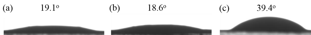
Fig. S4 Water contact angles of (a) EBC 750 , (b) EBC 800 , and (c) EBC 850
