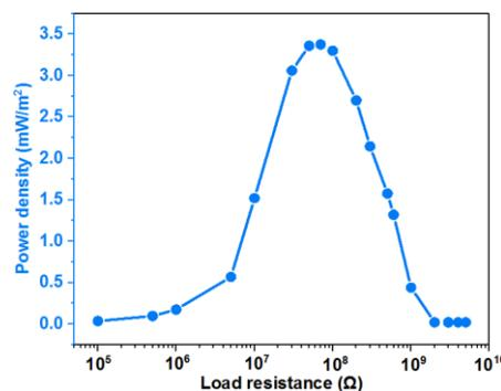
**Fig. S1** The dependence of power density on the external load resistance
