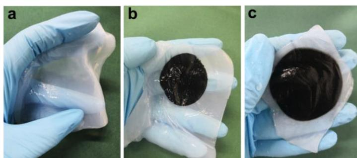
**Fig. S3** Images of (a) pure BC film, (b) Pt-Pd/MWCNTs/BC film and (c) MWCNTs/BC/MWCNTs film
