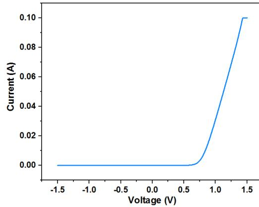
**Fig. S8** Rectification character of the used unilateral diode. When the applied voltage was between -1.5 V to 0 V, the current was near to zero. When the applied voltage was between +0.5 V to + 1.5 V, the current rapidly increased to amperes. This asymmetric I-V curve indicated a good rectifying ability of the unilateral diode, which can effectively prevent the reverse charging
