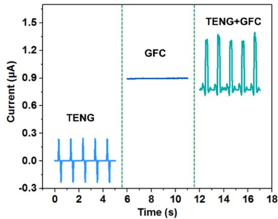
**Fig. S9** Output current of unrectified TENG, GFC, and their hybrid device
