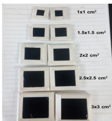
**Fig. S6** Independent GFCs with different sizes from  $1 \times 1$  to  $3 \times 3 \text{ cm}^2$  for performance test
