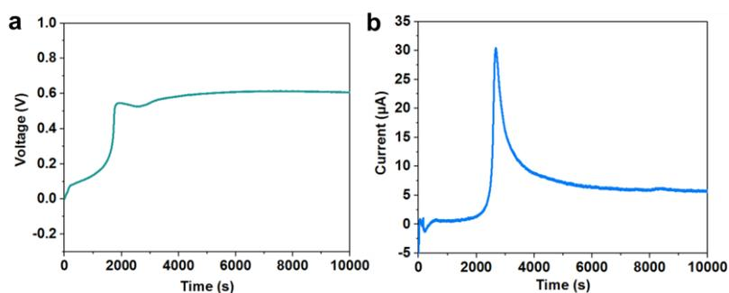
**Fig. S7** (a) A typical output voltage curve and (b) a current curve of GFC with a size of  $2 \text{ cm} \times 2 \text{ cm}$ . The voltage value and current value were obtained at its stable stage after  $5000 \text{ s}$  (e.g.,  $0.6 \text{ V}$  and  $6 \text{ µA}$ )
