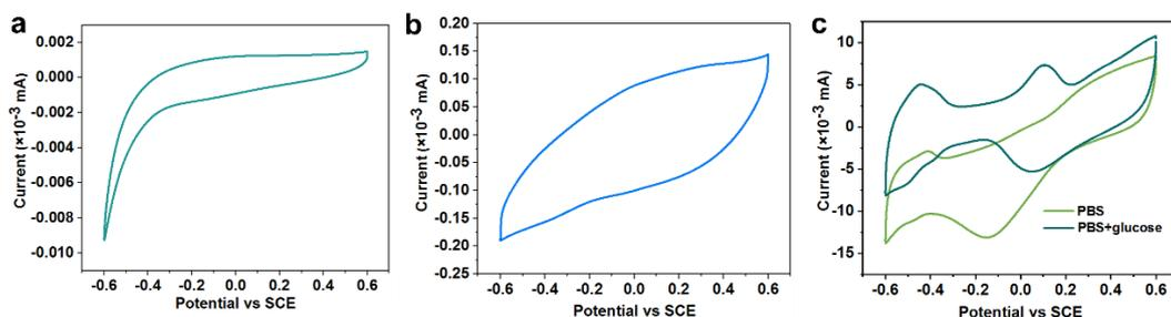
**Fig. S5** CV test of (a) pure BC film and (b) MWCNTs/BC film in PBS solution at  $10 \text{ mV s}^{-1}$  with glucose. (c) CV test of Pt-Pd/MWCNTs/BC film in PBS solution at  $10 \text{ mV s}^{-1}$  in the absence (green curve) and the presence (cyan curve) of glucose
