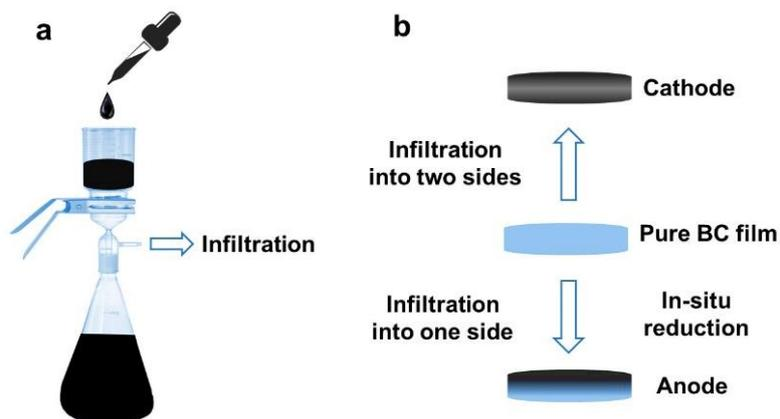
**Fig. S2** Infiltration diagram of cathode and anode of GFC
