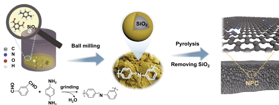
Fig. 1 Schematic representation of the preparation of N-doped porous carbon (NPC) via a mechanochemical route
