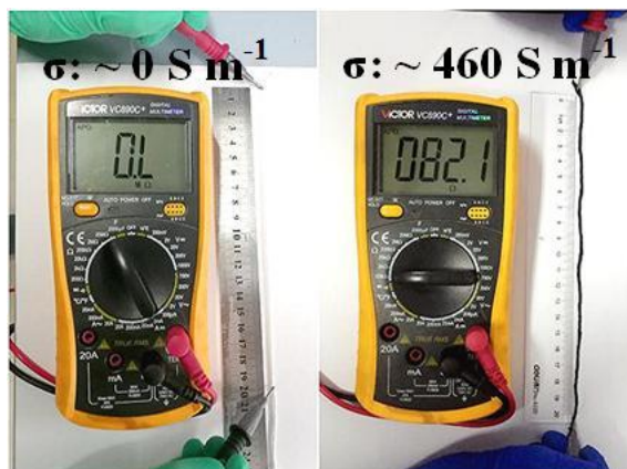
Fig. S14 Conductivities of pristine cotton yarn (left) and RGO/PEDOT modified cotton yarn (right)
