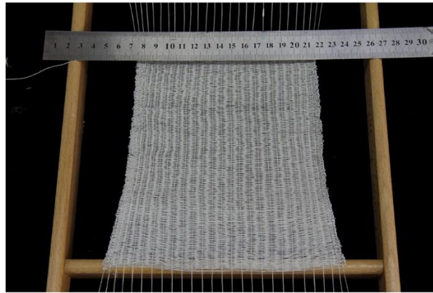
Fig. S9 Photograph of the SF/SSF yarn woven into large scale textile
