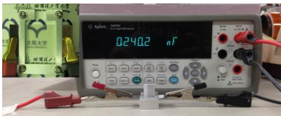
Fig. S8 The experimental setup of capacitance response measurement. Inset: Transparency of the capacitive pressure sensor involving both AgNW electrodes with transmittance of 93.7 % at 550 nm wavelength.
