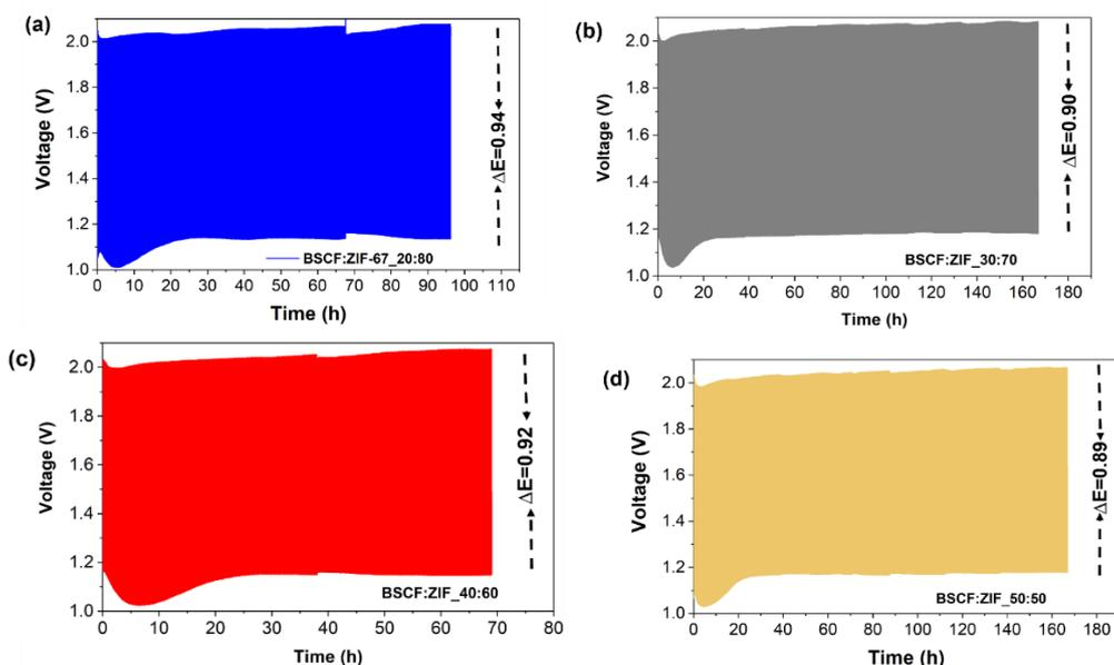
**Fig. S6** Galvanostatic charge/discharge test based on physical mixing of BSCF and C-ZIF-67 in different ratios (a) BSCF:C-ZIF-67\_20:80 (b) BSCF:C-ZIF-67\_30:70 (c) BSCF:C-ZIF-67\_40:60 and (d) BSCF:C-ZIF-67\_50:50 mixture catalysts tested for Cyclic stability at  $5 \text{ mA cm}^{-2}$
