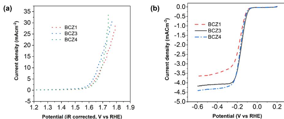
**Fig. S4** (a) OER and (b) ORR polarization curves of various samples including BCZ1, BCZ3 and BCZ4 composites, prepared by in situ growth of ZIF-67 crystals on BSCF in an oxygen-saturated 0.1 M KOH at a rotating speed of 1600 rpm
