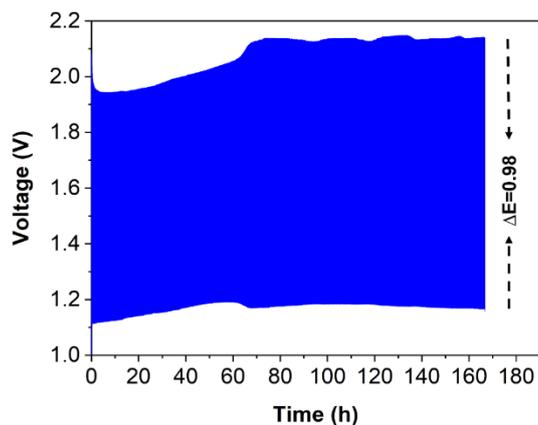
**Fig. S7** Galvanostatic charge/discharge test based on BSCF catalyst tested for cyclic stability at  $5 \text{ mA cm}^{-2}$
