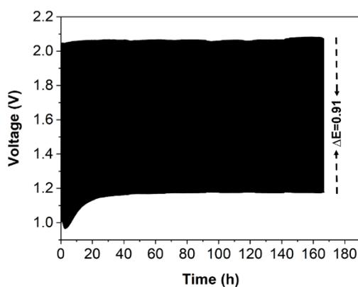
**Fig. S8** Galvanostatic charge/discharge test based on C-ZIF-67 catalyst tested for cyclic stability at  $5 \text{ mA cm}^{-2}$
