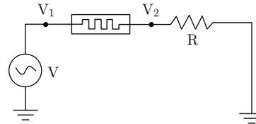
Fig. 3 Circuit diagram shows how  $I-V$  curve of the device was characterized.
