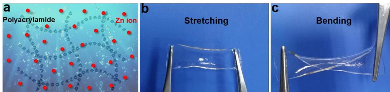
**Fig. S9** (a) Structural illustration, (b) and (c) optical images of the  $\text{Zn}(\text{CF}_3\text{SO}_3)_2$ -PAM hydrogel quasi-solid-state electrolyte
