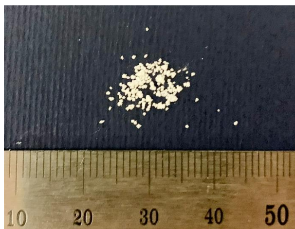
Fig. S10 Visual photo of BCP. They were particles, and each grid of the ruler was 1 mm
