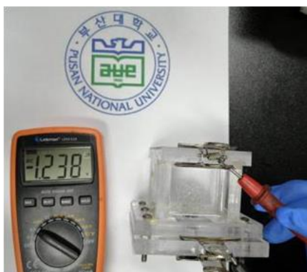
Fig. S15 OCV of used Zinc-air battery with Co-N 4 /NC after 100 cycles
