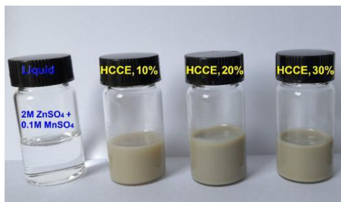
Fig. S2 Photographic images of liquid electrolyte and concentration colloidal electrolyte (HCCE, 10 %, 20 % and 30 %)
