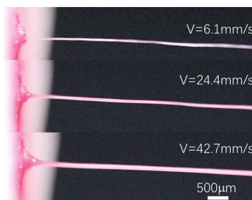
Fig. S4 Photographs of coating layer with different thickness formed on the silk fiber when using an oily-based ink (58.6 wt%) at different coating speed
