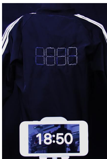
Fig. S14 Real display of digital fabric showing real time synchronized with mobile phone
