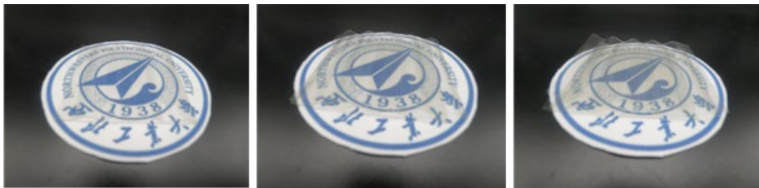
Fig. S3 The photographs of multilayered wavy PET/AgNWs/FEP composites with a good transparency: a Single layer. b Double layers. c Triple layers
