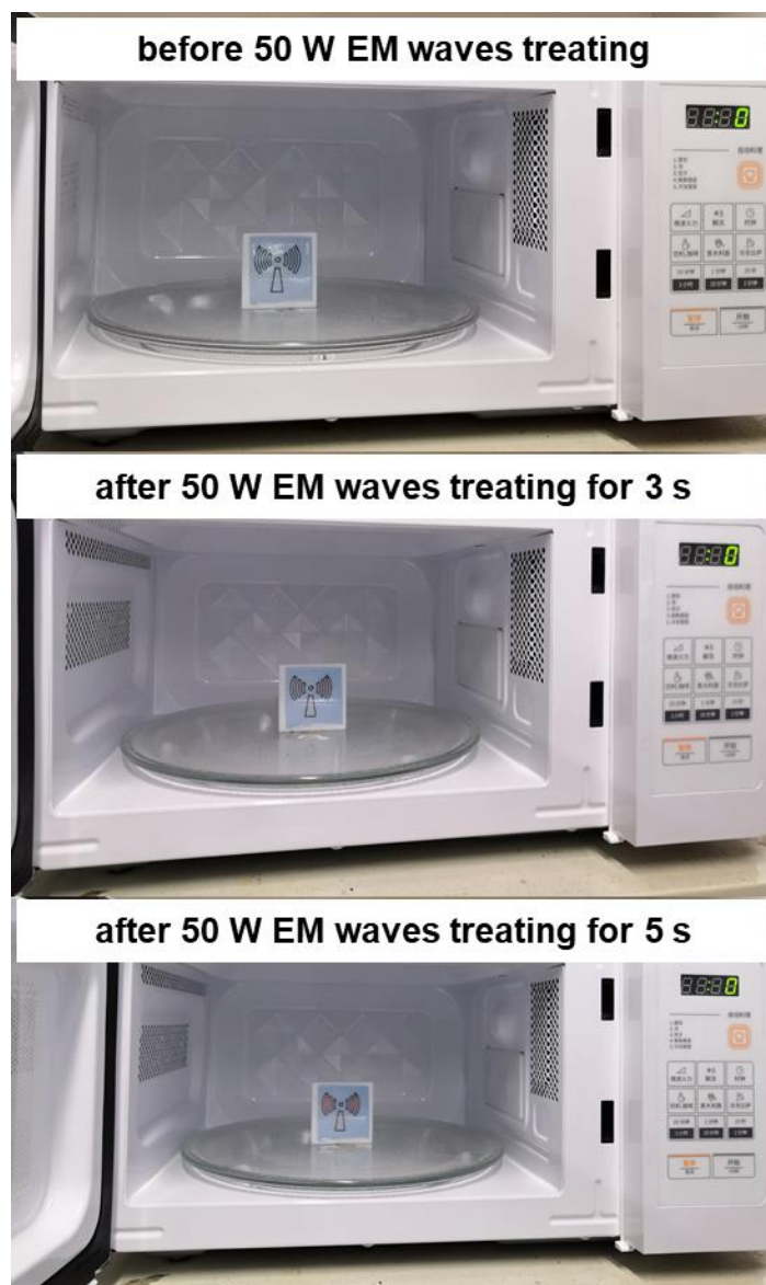
Fig S12. Color change of thermochromic MG3 under irradiation for different times in a microwave oven with a working frequency of 2.45 GHz.
