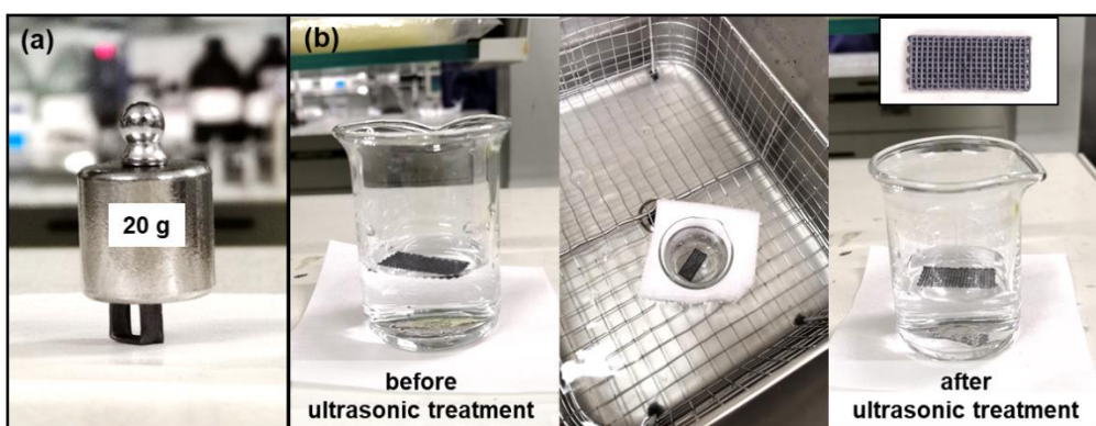
Fig S9. a Stable MG3 frame (6.8 mg) sustains a weight of 20 g. b Light MG frame floats on water, and there is no obvious structural change after ultrasonication at 240 W for 2 min.
