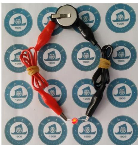
**Fig. S14** A red LED light with the working voltage range of 1.8 V-2.0 V driven by one half cell with MCS-7-900 electrode and K metal as counter electrode
