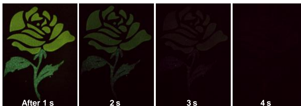
Fig. S19 Photographs of o-CDs@CA ink patterned flower after switching off the 365 nm UV lamp
