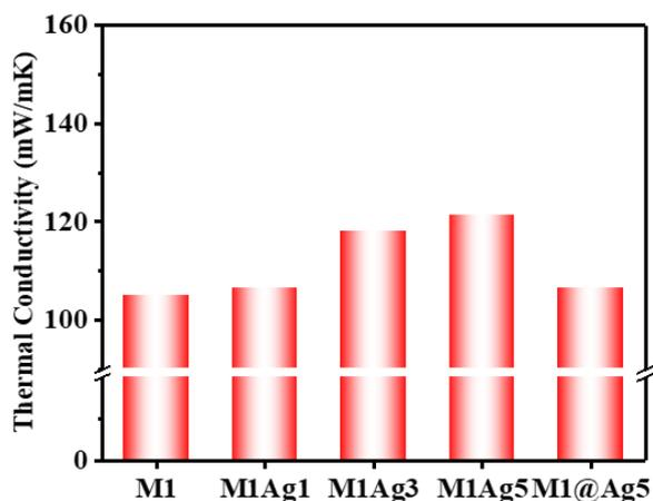
Fig. S7 Thermal conductivity of MxAgy EHF in through-plane
