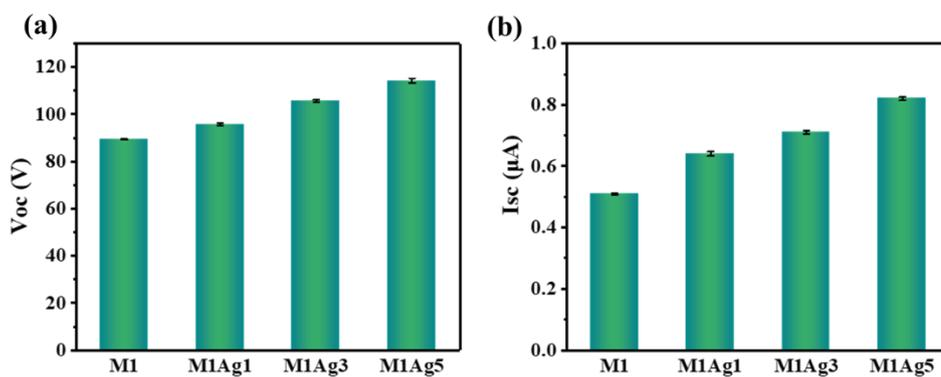
**Fig. S9** Variations in the **a**  $V_{oc}$  and **b**  $I_{sc}$  for MxAgy-based STENG with various AgMPs content at a frequency of 5 Hz and a force of 10 N
