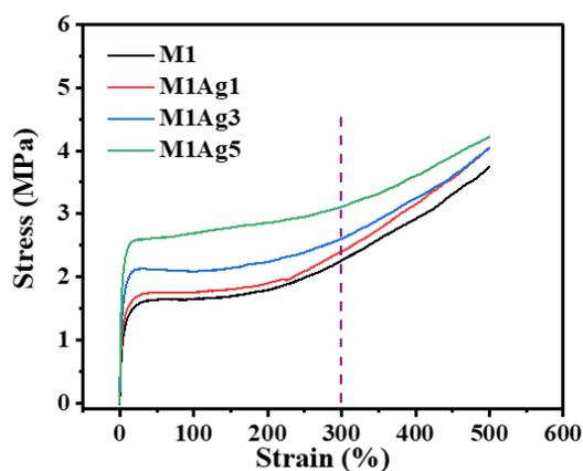
**Fig. S3** Typical stress–strain curves of the MxAgy EHF. The tensile strength increases due to the increase of AgMPs content and its embedding
