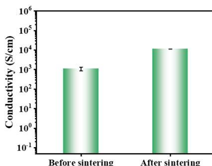
**Fig. S1** Comparison of electrical conductivity before and after hot-pressing
