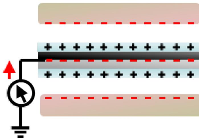
**Fig. S12** Electrical output mechanism of double triboelectric layers
