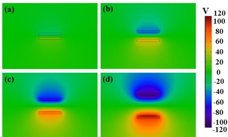
Fig. S8 Electrical potential distributions of the MxAgy-based STENG simulated by the COMSOL software
