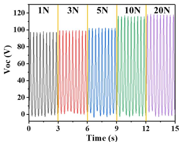
**Fig. S10**  $V_{oc}$  of the STENG with various applying pressure (fixed frequency of 5 Hz)
