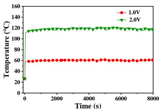
**Fig. S4** Electric-thermal property of M1Ag5 film at high and low temperatures for over two hours
