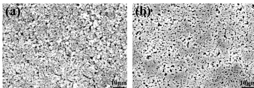
**Fig. S2** Micromorphology of AgMPs **a** before and **b** after hot-pressing
