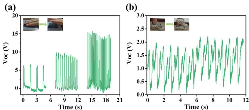
**Fig. S11** Corresponding  $V_{oc}$  of the MxAgy-based STENG to monitor **a** finger bending of different frequencies and **b** regular steps
