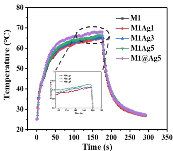
**Fig. S5** Temperature of different films under 100 mW cm<sup>-2</sup>
