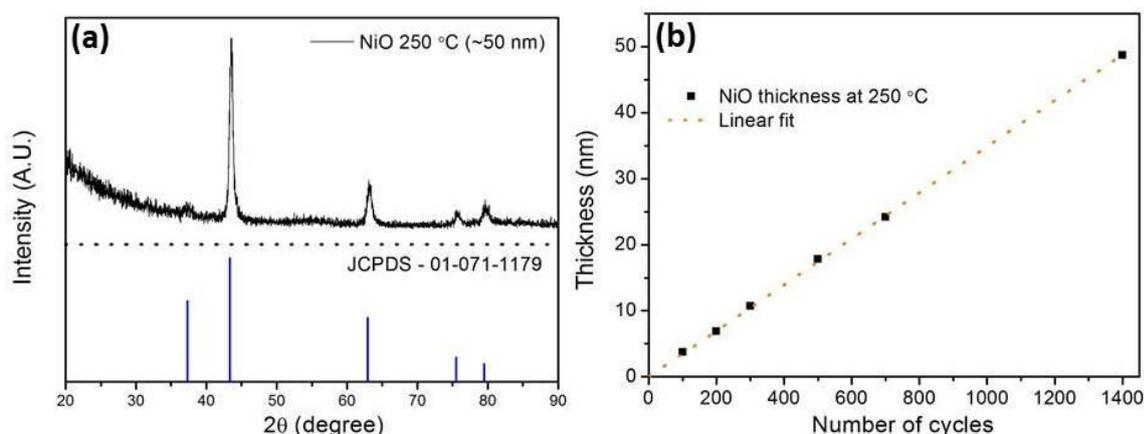
**Fig. S4** (a) XRD spectrum for NiO prepared by atomic layer deposition over the silicon substrate for 50 nm at 250 °C and (b) thickness versus cycle number for NiO at a reaction temperature of 250 °C
