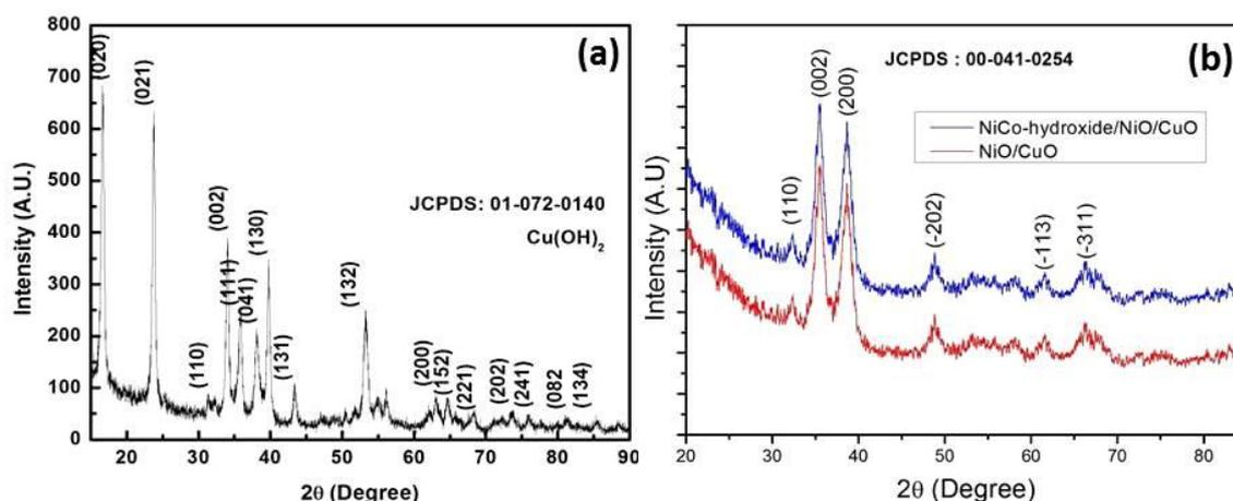
Fig. S2 XRD patterns of the prepared electrodes
