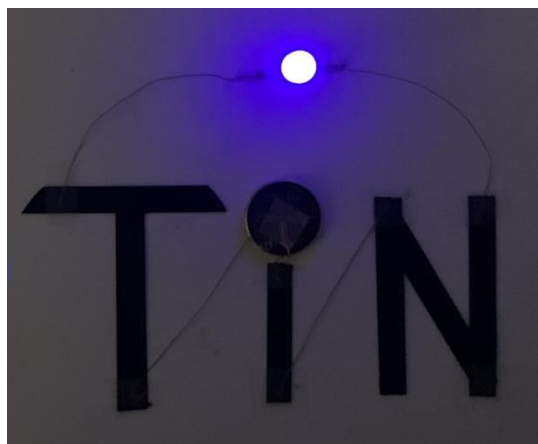
Fig. S7 A digital image of TiN papers as a part of the electrical connections to light a blue LED by a commercial 3V battery in dark environment
