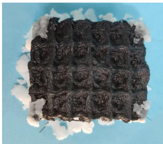
Fig. S23 The salt particles can easily fall off the edge from the evaporator under the action of external force
